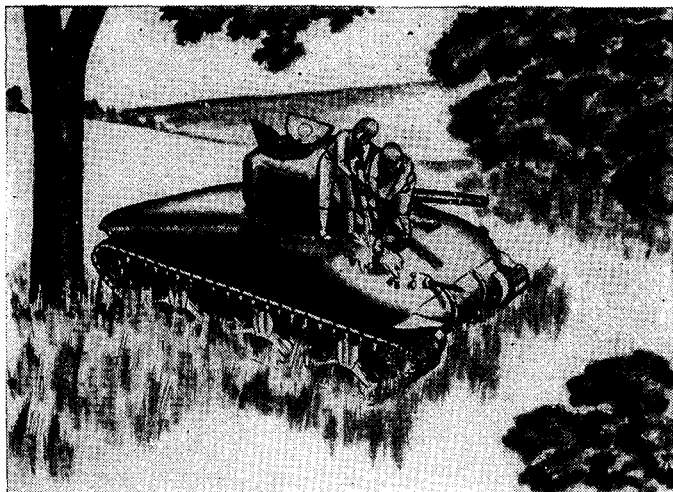
FIGURE 16.—Clean a path ahead of you as you descend so that you will not be contaminated by the gas drops or splashes on the vehicle.
